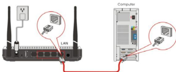
3. Connection between the Router and Network
