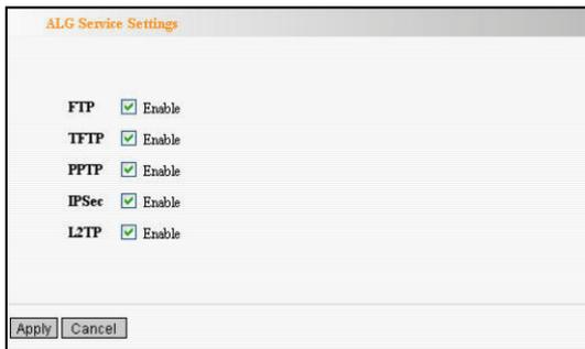
In order for these protocols to work through NAT or a firewall, either the application has to know about an address/port number combination that allows incoming packets, or the NAT has to monitor the control traffic and open up port mappings (firewall pinhole) dynamically as required. Legitimate application data can thus be passed through the security checks of the firewall or NAT that would have otherwise restricted the traffic for not meeting its limited filter criteria.
