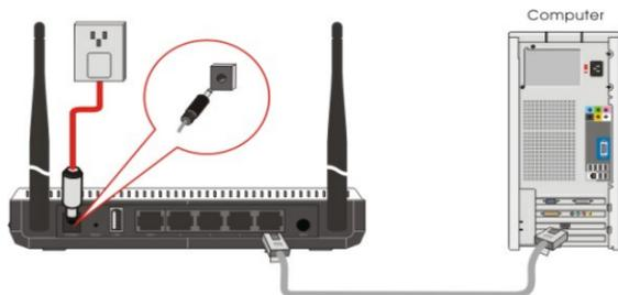
2. Please connect the LAN port of the Router to the network adapter of your computer with a cable.
